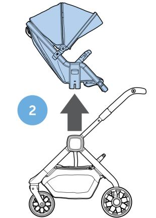
REMOVING SEAT / ENLEVER LE SIÈGE / SITZ AUSBAUEN / QUITAR ASIENTO / RIMOZIONE DEL SEDILE / USUWANIE SIEDZENIA
