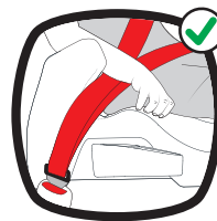
CORRECT SEAT BELT BUCKLE POSITION
