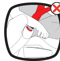
INCORRECT SEAT BELT BUCKLE POSITION
